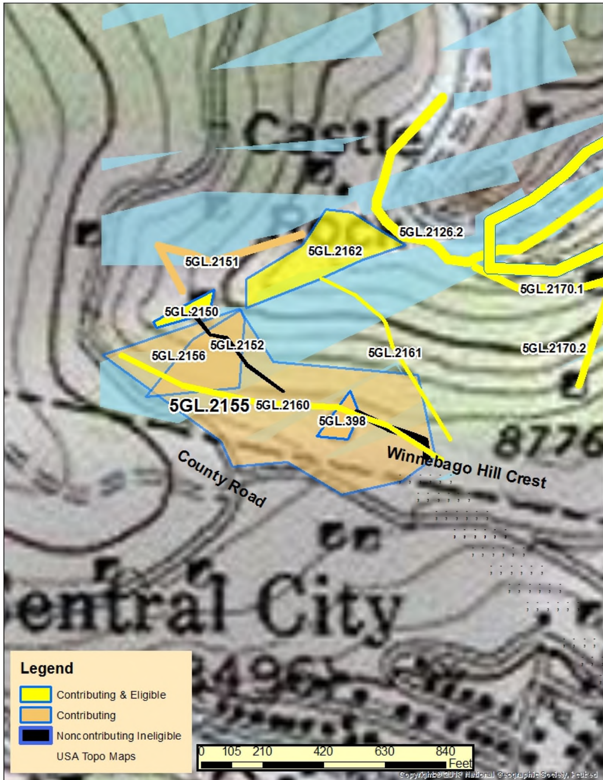
Figure 4.46: The large polygon at center on the topographic map enlargement (1:3,000 scale) is a GIS shape file illustrating Central City Dump's location and outline. The elongated blue wedges are BLM land tracts. The other polygons are mines superimposed over or adjacent to the dump. The yellow and black lines are linear resources.
