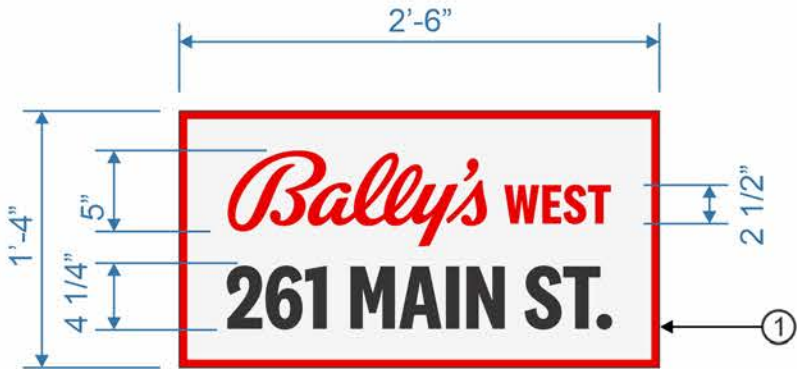
B.ID-5 NON-ILLUMINATED WALL PLAQUE SCALE @ 1" = 1'-0" QTY: ONE (1)
