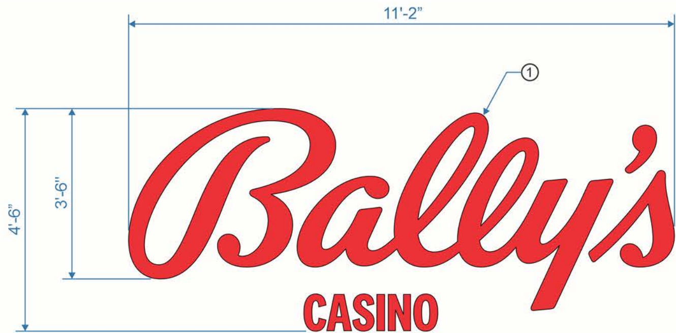
BG-8 ILLUMINATED CHANNEL LETTERS SCALE @ 1/2" = 1'-0" QTY: ONE (1) REQ'D
