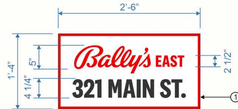
B.ID-8 NON-ILLUMINATED WALL PLAQUE SCALE @ 1" = 1'-0" QTY: ONE (1)
